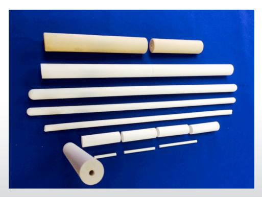
Proprietary compositions have been developed to facilitate core removal.
